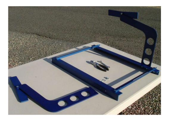
Install the right hand Upright Assembly to the outside of the right side of the Base Frame using 2ea. <sup>1</sup>/<sub>4</sub>-20 hex bolts, 2ea. lock washers, and 2ea. <sup>1</sup>/<sub>4</sub>-20 hex nuts. Make certain that the cradle is on the outside of the Upright Assembly. This will give you the maximum width between the cradles. Repeat this procedure for the left side again making certain that the Upright Assembly has the Cradle to the outside.
