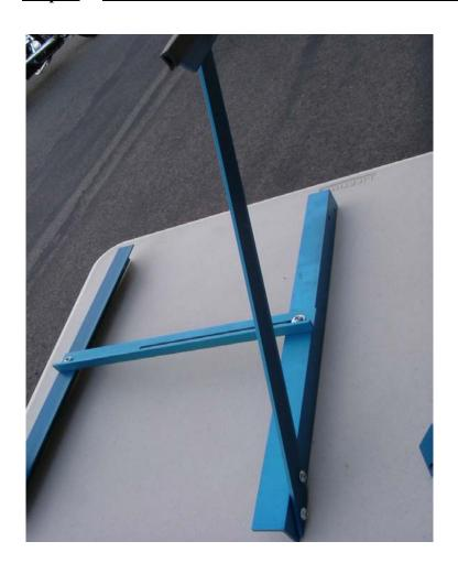
Install the right hand Upright Assembly to the outside of the right side of the Base Frame using 2ea. 10-32 bolts, 2ea. lock washers, and 2ea. 10-32 hex nuts. Make certain that the upright angles inward towards the center of the frame assembly and that the cradle is on the outside of the Upright Assembly. This will give you the maximum width between the cradles. Repeat this procedure for the left side again making certain that the Upright Assembly has the Cradle to the outside.
